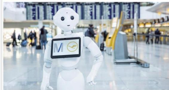
Josie Pepper's core contains a high-performance processor with WLAN internet access, which creates a connection to a cloud service where speech is processed, interpreted and linked to the airport data.
